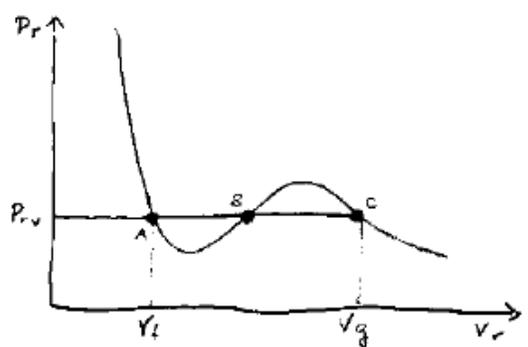
Point A =  $V_{rf}$  = smallest root
