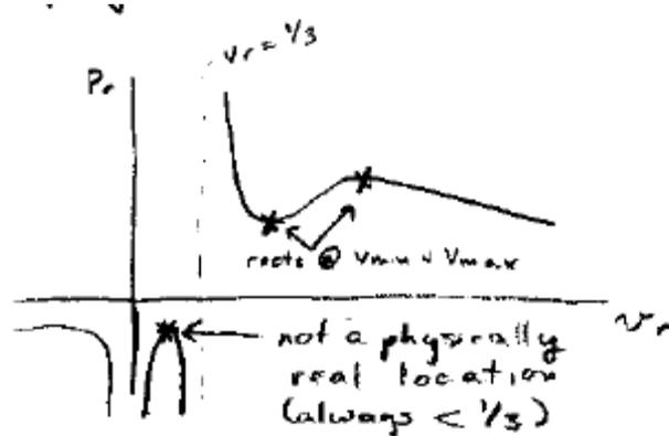
Once  $V_{rmin}$  and  $V_{rmax}$  are known, they are substituted back into (\*) to find  $P_{rmin}$  and  $P_{rmax}$ .
